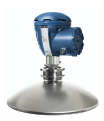
Rosemount 5900C with parabolic antenna is a non-contact radar level gauge. The parabolic antenna is the preferred antenna type for installation on tanks with fixed roofs without a still-pipe. It can be installed on existing manhole covers and close to the tank wall due to the narrow radar beam and the high signal to noise ratio. In certain cases, it can be used on tanks with floating roofs to measure the distance down to a target plate on the floating roof.
