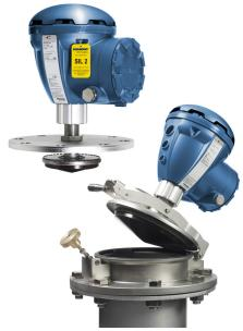
The Rosemount 5900C with array antenna is a non-contact radar level gauge for still-pipe measurement. It is available in two versions, Fixed and Hinged Hatch. Typical applications are crude oil tanks with floating roofs and gasoline/product tanks with or without inner floating roofs.
